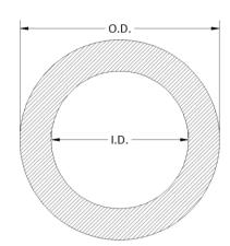
Find the outside diameter if T = 1.32 mm and I.D. = 14 mm.
