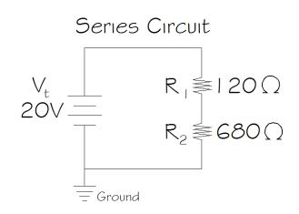
31. Use the Current Divider Formulas to calculate currents I<sub>1</sub> and I<sub>2</sub> at each resistor R<sub>1</sub> and R<sub>2</sub>.
