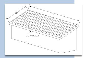
2. The formula for the area of a rectangle is A = LW. 74 ft x 38 ft = 2812 ft<sup>2</sup> this is the area of the roof  $2812 \text{ ft}^2 \times \frac{1 \text{ sheet}}{32 \text{ ft}^2} = 87.875 \text{ sheets}$  the area of one sheet of plywood is 4 ft x 8 ft = 32 ft<sup>2</sup>
