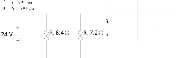
13. **Challenge Problem:** Fill in the table of values accurate to two decimal places for the electrical circuit wired in **series/parallel**, using the two primary electrical formulas:
