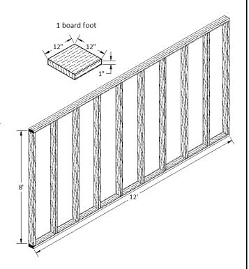
20. Lumber is often priced by the board foot. Calculate the number of board feet in 18 beams that are  $4'' \times 8'' \times 20'$ .
