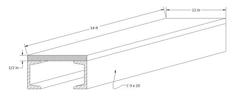
14. Use the steel design table in the appendix to find the weight of the welded steel platform to the nearest kilogram.
