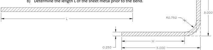
25. A piece of .375-inch thick sheet metal is to be bent at 135° to the finish dimensions shown. All measurements are in inches. Use the formulas from question 23.
