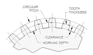
Working Depth = .6366 x Circular Pitch Clearance = .05 x Circular Pitch Tooth Thickness = .5 x Circular Pitch
