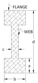
Note: Moment of inertia is a measure of a beam's effectiveness at resisting bending based on its cross-sectional shape.
