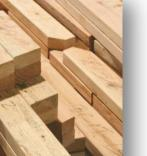
Note: Although the dimensions are actually  $1\frac{1}{2}^{\frac{1}{2}}$  x  $3\frac{1}{2}^{\frac{1}{2}}$ , the nominal measurements 2" x 4" are used in the calculation of board feet.
