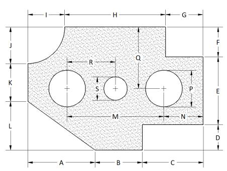
6. Measure the dimensions A through S on the part to the nearest 32<sup>nd</sup> of an inch. Answer as a reduced fraction.
