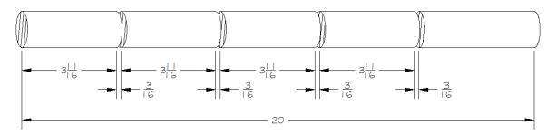
18. A length of round stock is to be cut into six equal lengths using a saw that removes 3/8" with each cut. Calculate the length of the equal piece. All dimensions are in inches.
