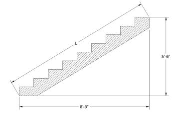
6. Stair railings have spindles that are required by code to have no more than a 4" space between them. If the slope of the stairs causes the height of adjacent spindles to differ by 3", calculate the distance the 1" wide spindles are apart <u>along</u> the handrail so that the holes can be drilled.
