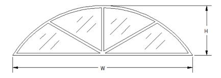
Find the radius of an arch window accurate to the 16<sup>th</sup> of an inch, which has a width of 42 inches and a height of 12 inches.
