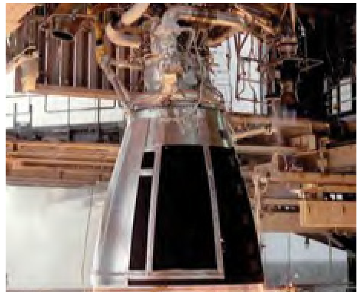
RS-68 Liquid propellant engine test firing.
