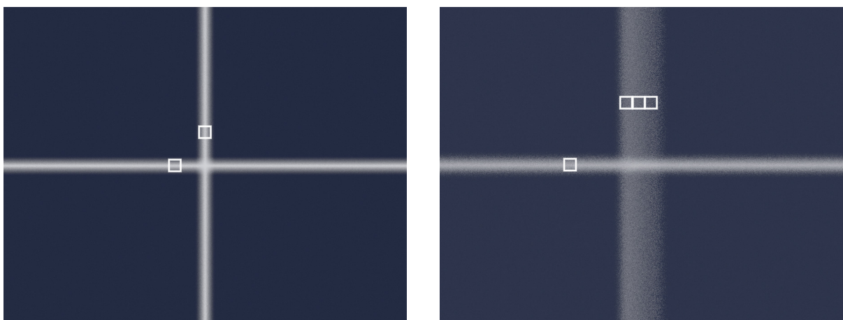
Fig. 12: Beam spread of the concentric spherical display at center (left) and with the eye camera turned right 20^\circ around the pupil position, assessing the eye peripheral resolution (right). Squares of 1 arcmin x 1 arcmin are overlaid for comparison. The grid lines displayed are originally <1 arcmin wide.
