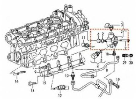
Figure 1. The high pressure fuel pump.
