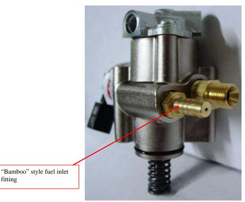
FIG 2: FSI Fuel Pump shown with "Bamboo" type fitting where a hose is pushed-on to the barbed fitting and secured with a hose clamp.
