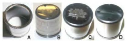
Figure 2. Cam followers in various stages of wear: holed base (A), excessive wear (B), normal wear (C), and new part (D).
