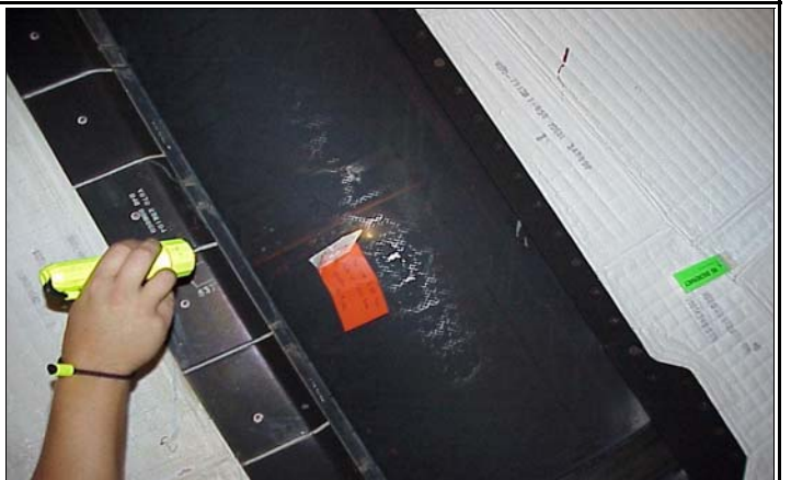
Figure 3. Overview of the STS-92 vertical stabilizer impact area.
