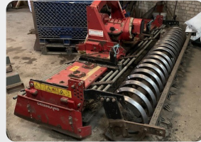
GREENLAND 3M POWER HARROW Reference Number: 15547 c/w 3M working width, flex coil & star cleaner. (JI)
