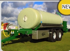
NEW BAILEY 15000 LITRE WATER BOWSER Reference Number: 12167 1000L/min pump on 3" outlets, 2x extra long 3" hoses (JP)
