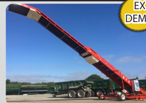
SWIFTLIFT 900 EXTENDO ELEVATOR Reference Number: 9034 c/w 3 phase electrics, variable speed, auto slewing platform (DD)
