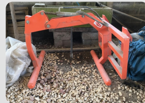
RITCHIE SILAGE GRAB Reference Number: 13508 c/w JCB Q fit fittings, hydraulic over the top grab arm. (DD)
