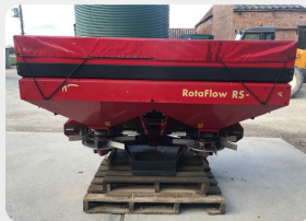
VICON ROTAFLOW RS-L FERTILISER SPREADER Reference Number: 15551 c/w - 800 litre hopper with extensions, 8 vanes per disc (JP)
