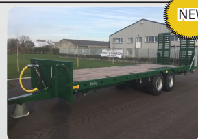
NEW BAILEY 15T LOWLOADER Reference Number: 12166 c/w hyd. brakes, parking brakes, strap points, heavy duty EN8 towing eye, hardwood floor.
