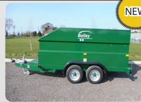
NEW BAILEY 2000L FUEL BOWSER Reference Number: 10169 c/w high speed running gear, mudguards, brakes, screw jack/ jockey wheel (JP)
