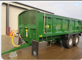
BAILEY 14T ROOT TRAILER (2020) Reference Number: 14644 c/w hyd. door, sprung drawbar, 1900mm track, 3'9" sides, easy sheet, grain chute, air and oil brakes.
