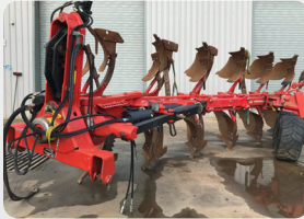
5 FURROW GREGOIRE BESSON PLOUGH (4+1) Reference Number: 15409 C/W 4+1, 160hp Headstock, 90cm Point to point (BF)
