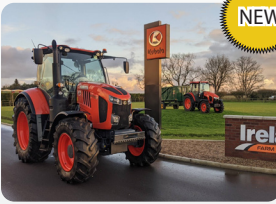
KUBOTA M7152 Reference Number: 14769 c/w 50k powershift gearbox with creep, front suspension, air trailer brakes, cab suspension (JP)
