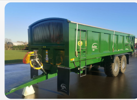
BAILEY 16T ROOT TRAILER (2020) Reference Number: 14490 c/w hyd. door, sprung drawbar, 1900mm track, 3'9" sides, front flaps, air brakes.
