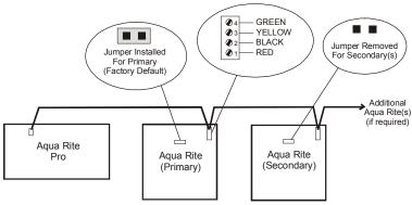
NOTE: Primary/Secondary jumper is located underneath small circuit board.
