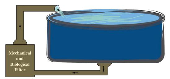
Figure 6. Example of recirculating system, which recycles its water by passing it through a series of biological, mechanical and sometimes chemical filters to remove waste and excess nutrients.
