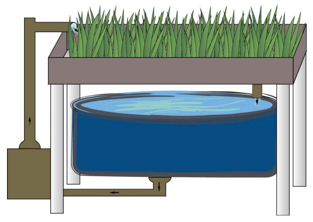
by bacteria in the water/filter that the plants can then use to grow. The plants act as a filtration system for the fish.
