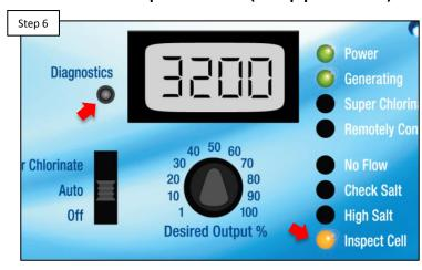
IF the "Inspect Cell" LED was flashing alone, press and hold the diagnostics button for 5 seconds OR until the Inspect Cell LED goes out. This will reset the inspect cell timer for another 500 operational hours.
