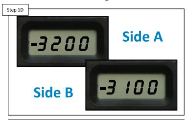
Reset the average salt level, twice, following the steps on pg. 10. Are the two instant salt level readings within 500ppm of each other? IF not go to step 1E. IF they are go to step 1F.
