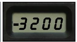
Press Diagnostics button 5 times to display the Instant Salt level.
