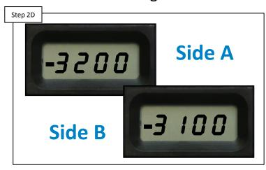
Reset the average salt level, twice, following the steps on pg. 10. Are the two instant salt level readings within 500ppm of each other? IF not go to step 2E. IF they are go to step 2F.
