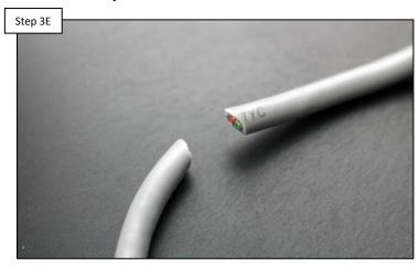
IF the flow switch wire is damaged, the signal will be interrupted so replace the flow switch (GLX-FLO-RP). IF the wire is not damaged, proceed to step 3F.
