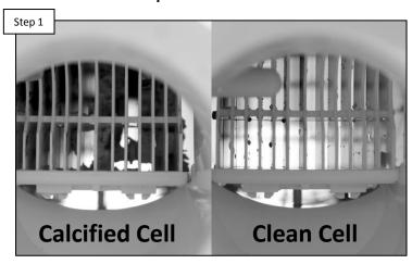
Holding the cell up to a light source, inspect for calcium deposits. Even if a TurboCell appears clean, it may still require cleaning if salt accuracy is off AND/OR chlorine production has diminished.
