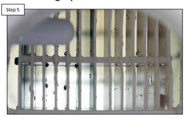
After the solution has been safely removed, thoroughly rinse the TurboCell before returning it to its place in the plumbing. Once returned turn the pump back ON and proceed to the step 6.
