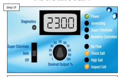
IF the "Check Salt" & "Inspect Cell" LEDs cleared, then the problem is solved. IF not please contact technical support directly by dialing: 908.355.7995 or email support via Hayward.com's support page.
