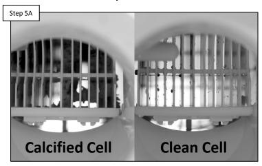
Inspect the cell for calcification. Clean the cell & reset the average salt reading (pg. 10). IF the message still appears AND the water temperature is not greater than 139F or lower than 51F, then go to 5B.
