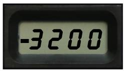
When the instant salt level is stable (and the negative sign still present), slide switch to 'Super Chlorinate' and back to 'Auto'.
