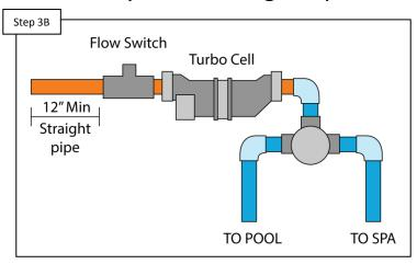
It is recommended for the flow switch to have 12" of straight pipe preceding it (the TurboCell counts as straight pipe). IF not, consider moving the flow switch.
