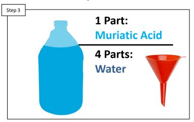
Mix a solution comprised of 4 parts water to 1 part Muriatic Acid. <u>Always Add Acid to Water</u>. Once mixed turn the turbo up vertically either in a bucket or using the recommended cell cleaning stand.
