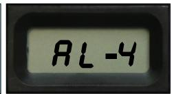
When the unit reads 'AL-4' move the switch up to 'Super Chlorinate' and back to 'Auto'.
