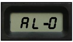
Continue moving the switch up to 'Super Chlorinate' and back to 'Auto' until the display reads 'AL-0'.
