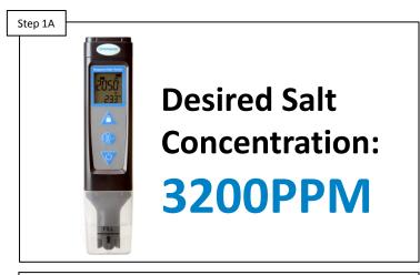
Test the salt concentration of the water using an independent test, with a calibrated salt meter. If the salt level is below 3200, raise the salt level (referring to salt addition table pg. 30). IF fine, go to 1B.
