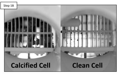
The TurboCell must be clean in order to report accurate salt readings. IF the cell looks like the image on the left, clean the cell (pg.12-14). IF cell is clean, proceed to step 1C.
