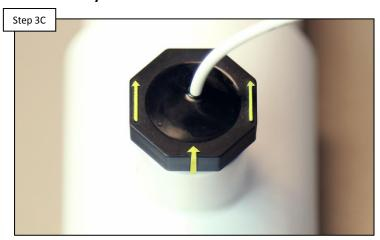
Verify the arrows (located on switch top) are pointing in the same direction water is flowing. IF incorrect, rotate the switch until it matches the direction of water flow (DO NOT OVERTIGHTEN). IF correct go to 3D.
