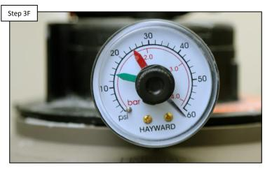
Check Filter pressure & pump basket for debris.
