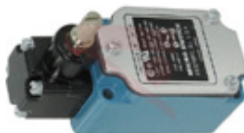
△ Limit Switch A121705 SPDT, 1 NC/1 NO. 10 Amp. Snap Action. Provides warning for Tank Up, Boom Up, Load Limit, and Door Lock.
