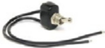
△ Toggle Switch A120180-1 SPST, Off - On. Plasticized 2 wires, 25A@12VDC. Typically used for floodlight application
