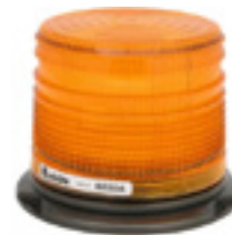
△ Low Profile, High Intensity Amber Strobe A338716 12-24V, 72 Quad FPM. 6.375" Dia. Base X 5"H Compatible with all models.
