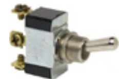
△ Toggle Switch A120861-3 SPDT, On - On. 3 screw terminals. 25A@12VDC. For Rear Panel Blower & Water Pump
