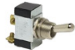
△ Toggle Switch A120859-1 SPST, Off - Mom. On. 2 screw terminals, 25A@12VDC, Boom Flapper Switch
