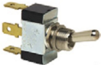
△ Toggle Switch A120861 SPDT, On – On. 3 blade terminals, 25A@12VDC. Cab Blower, PTO and Water Pump switch.
