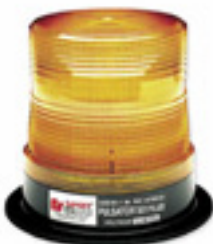
△ High Profile, High Intensity Amber Strobe A380028 12-48V, 80 FPM. Dual Flash. 6.5" OD X 6"H. Advanced Lens Optics. Compatible with all models.
