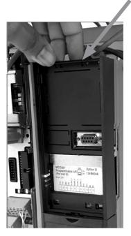
Carefully remove the plastic cover by unlocking the tab on the top of the drive and releasing.
