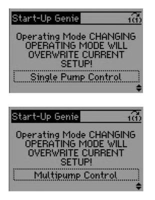
Select either Single Pump or Multi-Pump Control. Follow the programming for single pump application below.
