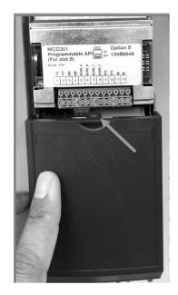
Carefully remove bottom cover by unlocking tab
