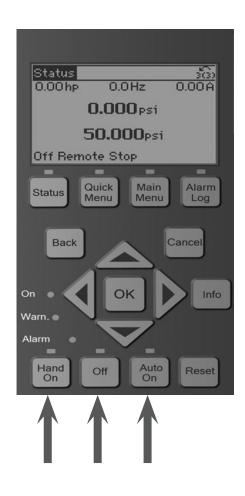
Check Pump and Motor Rotation by selecting Hand On. If motor is running backwards, power down drive, wait five minutes, and rotate motor wires from the drive. Once rotation is verified, select Off.
