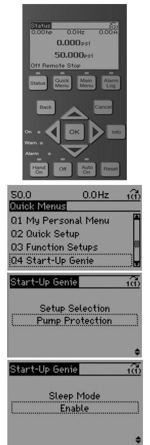
The No Flow Power Calibration Setup provides the method to program the no flow power curve in to the controller
