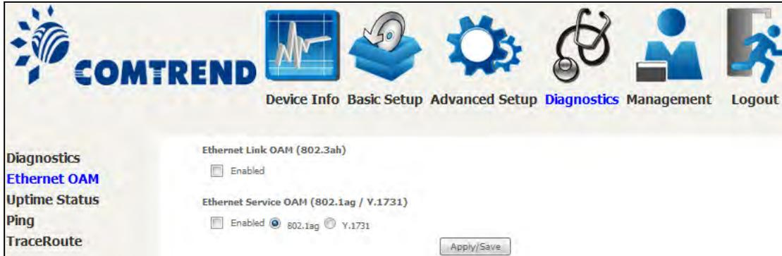
To enable Ethernet Link OAM (802.3 ah), click Enabled to display the full configuration list. At least one option must be enabled for 802.1ah.
