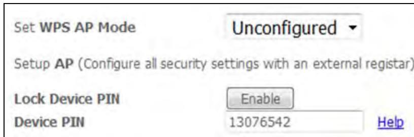
**Step 4:** Activate the PIN function on the wireless client. For **Configured** mode, the client must be configured as an Enrollee. For **Unconfigured** mode, the client must be configured as the Registrar. This is different from the External Registrar function provided in Windows Vista.
