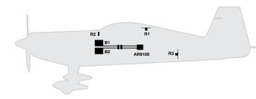
• 40% aerobatic plane with dual LiPo batteries, dual regulators and four remote receivers
