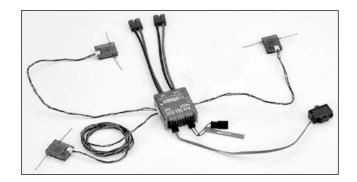
1. Using foam or thick double-sided foam tape and tie wraps, secure the main PowerSafe unit in the position that you would normally mount the receiver.
