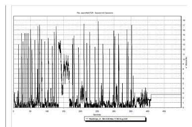
In the example above, the average current was 2.62 amps, which calculates to 435mAh per 10 minutes (typical flight length). It's recommended that only 60% of the available capacity be used to ensure plenty of reserve battery capacity. In this example using two 4000mAh batteries (8000mAh total capacity) x 60%= 4800mAh (available usable capacity) divided by the capacity used per 10-minute flight, 435mAh would allow up to 11 flights, of 10 minutes each.
