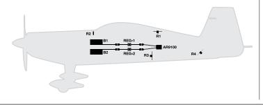
• Jet with dual LiPo batteries, dual regulators and four remote receivers
