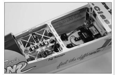
2. Mount the switch on the side of your aircraft and insert the switch plug in the port in the main unit marked SWITCH.
