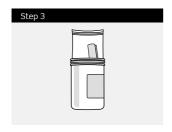
If the data logger is available, insert it inside the plastic container next to the sealed plastic bag.
