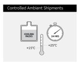
• To maintain **controlled ambient** (+15C to +25C) you need to pre-condition an adequate number of cooling packs by placing them in a **refrigerator** on a horizontal and flat surface for a minimum of 24 hours.
