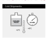
To maintain cold temperatures (+2C to +8C) you need to pre-condition an adequate number of cooling packs by placing them in a freezer on a horizontal and flat surface for a minimum of 24 hours.
