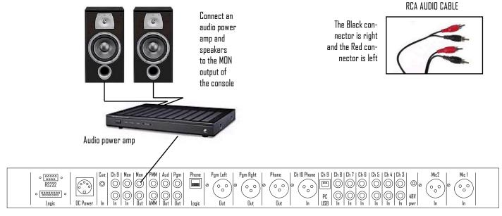
Back panel Diagram for ARC-10U (unbalanced base model) & ARC-10UP (unbalanced with PC model)
