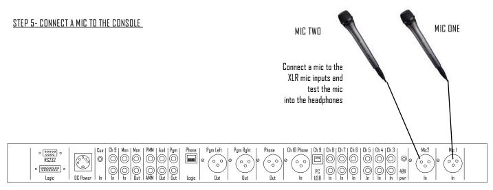
Back panel Diagram for ARC-10U (unbalanced base model) & ARC-10UP (unbalanced with PC model)
