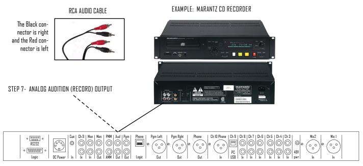
Back panel Diagram for ARC-10U (unbalanced base model) & ARC-10UP (unbalanced with PC model)
