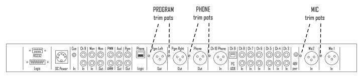
Back panel Diagram for ARC-10U (unbalanced base model) & ARC-10UP (unbalanced with PC model)
