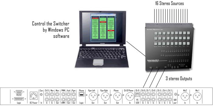
Back panel Diagram for ARC-10U (unbalanced base model) & ARC-10UP (unbalanced with PC model)
