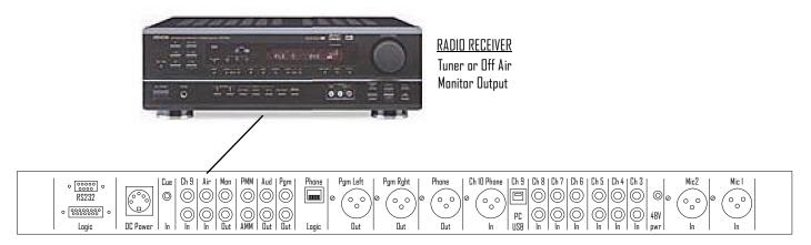
Back panel Diagram for ARC-10U (unbalanced base model) & ARC-10UP (unbalanced with PC model)
