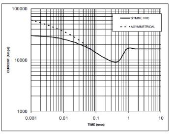
Some analysis programs account for decaying generator current in arc flash incident energy calculations Arc Flash EX #1 – Generator Source reduce to 300% of rated current after 5 cycles – Recalculate Trip Time Using Reduce Current
