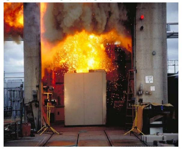
Arc Resistant Switchgear Undergoing Test For an Arcing Fault.
