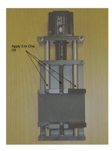
Whenever possible remove the consumable dust from the mechanical assembly of the height control. This works best with a compressed air nozzle.
