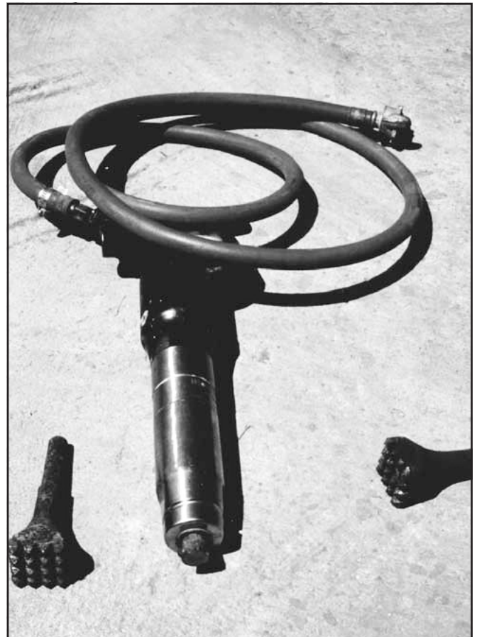
Figure 8-5. Tool used for bush hammering concrete surface
