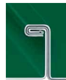
90° Field Seam Spanlok hp , Curved Span-Lok
