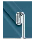
180° Field Seam SpanSeam
