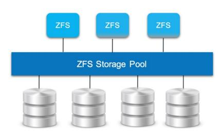
Figure 4: Graphical representation of ZFS pooled storage model.
