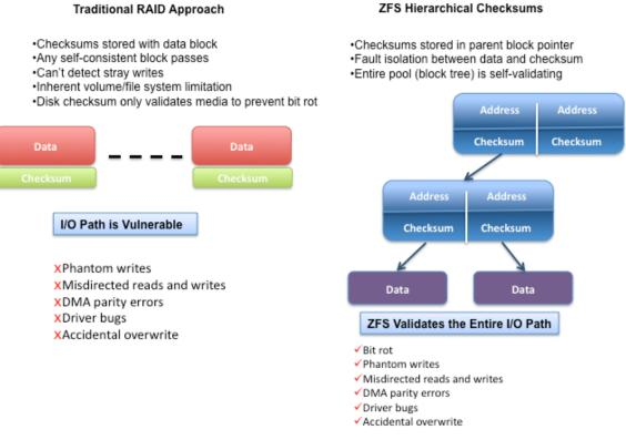
Figure 7: Description of ZFS hierarchical checksums versus traditional RAID approach.
