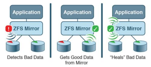
Figure 6: Example of how ZFS self-healing architecture corrects a corrupted block.
