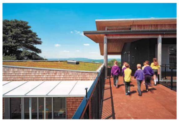
Ysgol Trimsaran (a school in Wales designed by Architype) used a locally sourced timber frame construction. It is Passivhaus certified and the first year of post-occupancy monitoring showed Ysgol Trimsaran to be using less than half of the primary energy of a comparison school designed to meet building regulations only Photo: Phil Boorman for Architype
