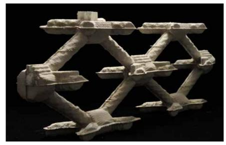
Steel fibre reinforced ultra-high performance concrete lattice. Non-standard prototype by Melika Aljukic. From *Mixed Matters: Concrete* by Melika Aljukic, Architectural Association, ILEK, str.ucture GmbH Stuttgart, 2016. Collection of the Institute for Lightweight Structures and Conceptual Design (ILEK), University of Stuttgart
