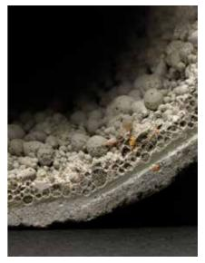
Controlled segregation of a non-standard concrete element at ILEK. Source: ILEK
