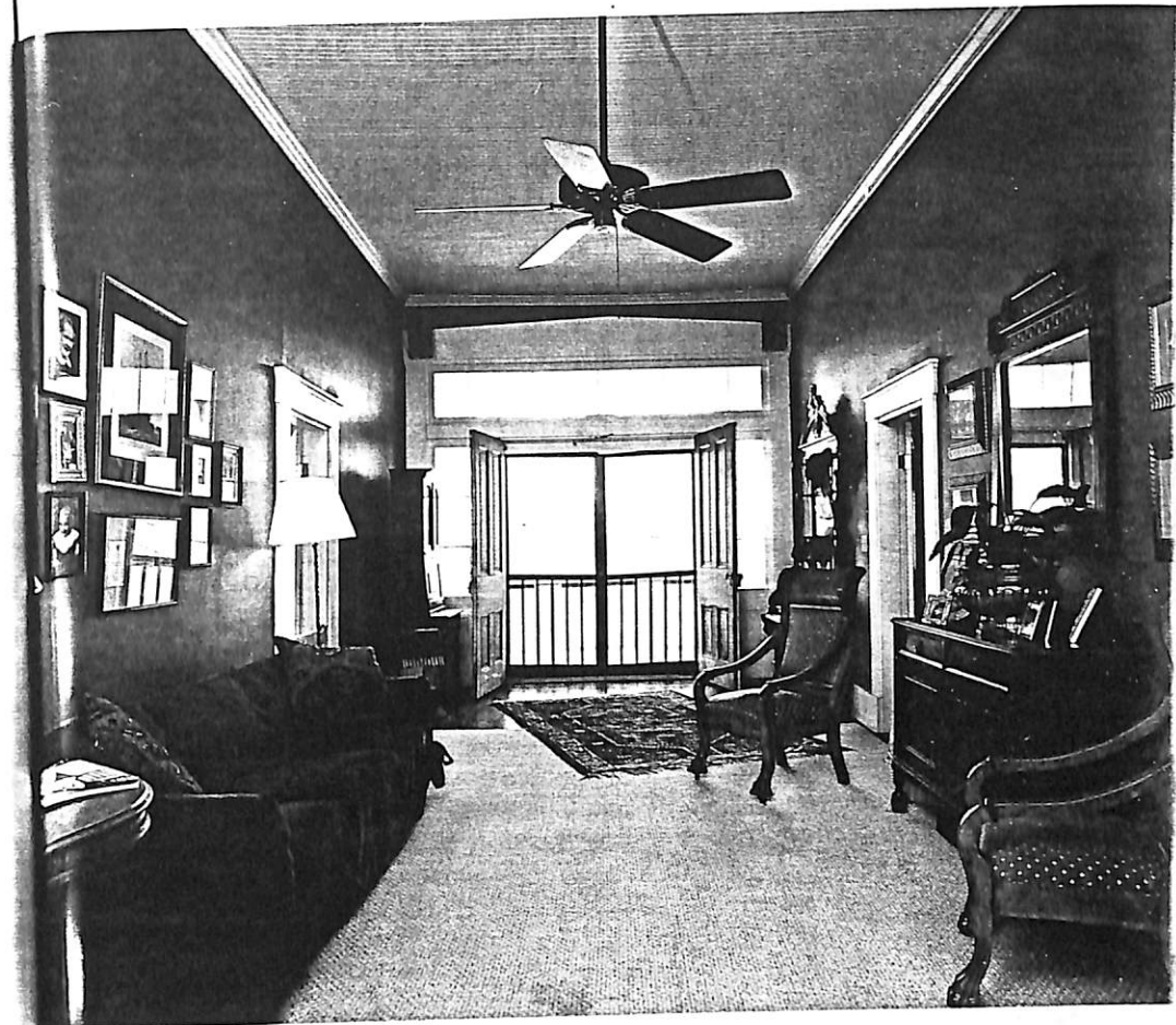
The P-Line house's center hallway opens onto a front gallery through double leaf doors with horizontal transom and sidelights. The nearby secretary, left, and hall tree, right, are original. The hardwood hall flooring is pine.
