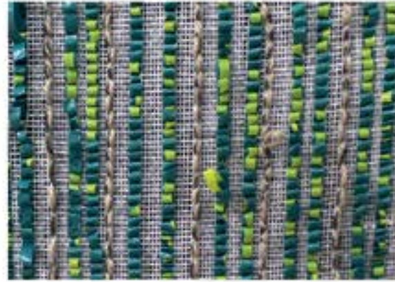
Alternate rows of conductive and plastic loops. (back of textile)
