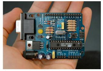
**Figure 1.** A serial Arduino board with removable Atmega8 microcontroller, one of the original versions of the Arduino hardware.
