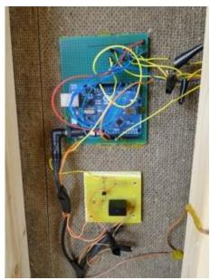
I built the first relay circuit from scratch. The circuit diagram is available in the Arduino inventors kit, but I don't recommend this route. In the second system, not only was it much more organized, but I also found a better solution to the relay circuit, our CPS156. I also used an Arduino ProtoShield instead of a bulky eurocard (see below).
