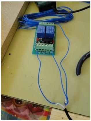
Then connect the positive terminal of the power supply to the positive connection on your electronic door strike. Connect the negative connection on the door strike to the normally open (NO) terminal block on the CPS156. The build is now complete. Now you are ready to configure the sketch and install in on the Arduino.
