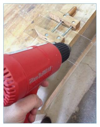
FIGURE 4.16 Using a heat gun to soften acrylic.
