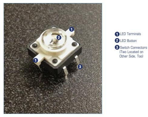
FIGURE 4.9 The button you use in the project has six connectors.
