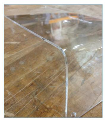
FIGURE 4.15 Bending acrylic is easy and gives a nice effect!
