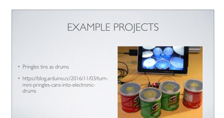
Vibration sensors in the Pringles tins go to an Arduino, which converts that to MIDI signals on the drum channel.
