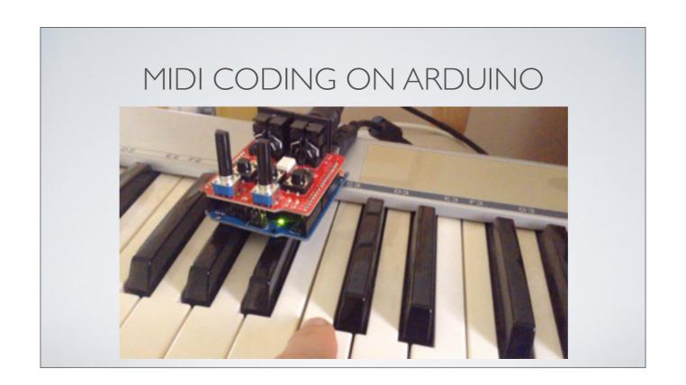
OK, so this is just flashing a few LEDs, and there aren't as many output pins on the Arduino as there are notes on the keyboard. What to do? We can use a chip called a shift register - it uses 3 pins from the Arduino to control 8 output pins. You can chain them together to get more output pins. Cost is about \$1 for 74HC595. There is an Arduino tutorial called ShiftOut that covers all of this.
