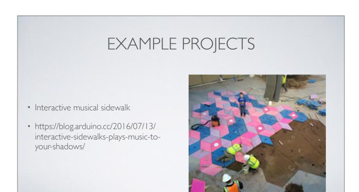
A large installation in Arizona - shadows trigger light sensors embedded in the ground, which goes to one of 6 Arduino controllers, which then interface with music software.
