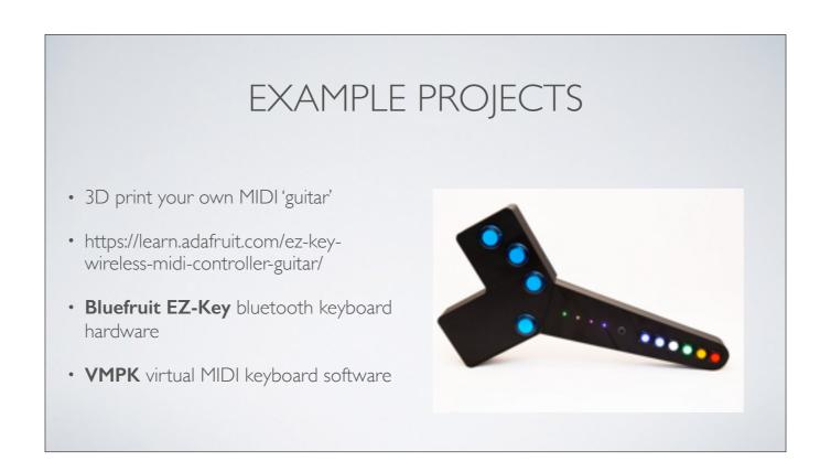
This is a different way to get MIDI from your build to your computer. The device has a bluetooth keyboard that sends ascii keys when you interact with the instrument. The computer is then running software to map those keyboard presses into MIDI messages, to send to Garage Band, etc.
