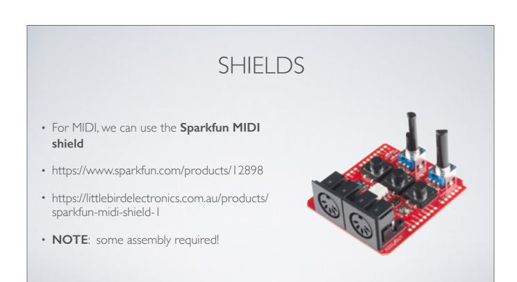
This shield has MIDI in and out connectors, 3 buttons to do stuff, and two variable resistors (the turny knob things) so you can vary things and use that to affect the MIDI signals, like volume, pitch, etc. There are other MIDI shields that just have the MIDI connectors, and don't have all the extra buttons and knobs, which you don't \*really\* need.
