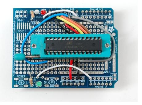
With the USB cable still plugged in (and the same Serial port selected as before) Select **Tools→Burn** Bootloader→w/Arduino as ISP
