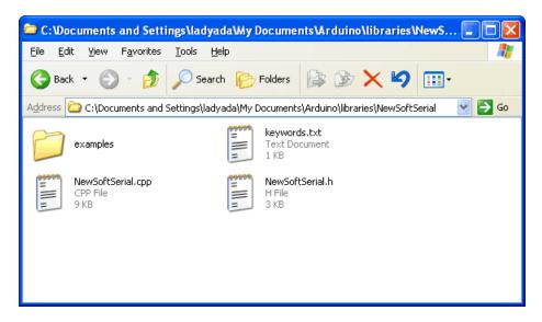
There may also be some **.o** files. The **.o** files are C++ compiled Objects. If you end up working on the library and modifying it, be sure to delete the **.o** files as that will force the Arduino IDE to recompile the modified **.cpp**'s into fresh **.o**'s.
