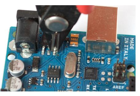
Then you'll need to heat the tab up to get it liquid so you can lift off the old part. Although it may seem counter intuitive, its best to **add** some solder to the tab, melt it on with your iron, this will improve the heat conduction since the tab is so large.
