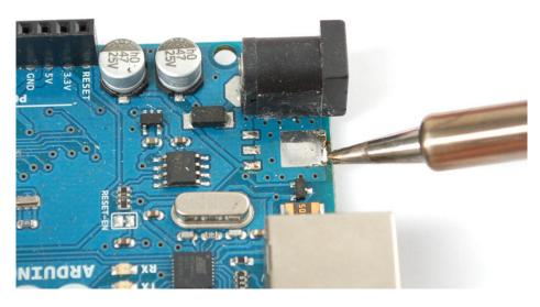
Now line up the new 3.3V regulator, and solder the tab first, use plenty of solder and be patient, the tab acts like a heat sink.
