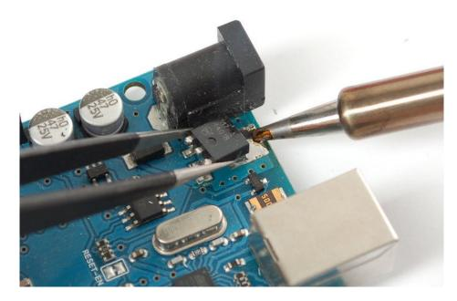
Clean up the tabs and remove any clipped parts still stuck on.
