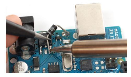
That's it! You are now 3.3V powered. This is a little lower than the power/frequency specification for the AVR chips since they ought to have about 3.6V to run 16Mhz but its *probably* not going to be an issue since AVRs can be overclocked a little.
