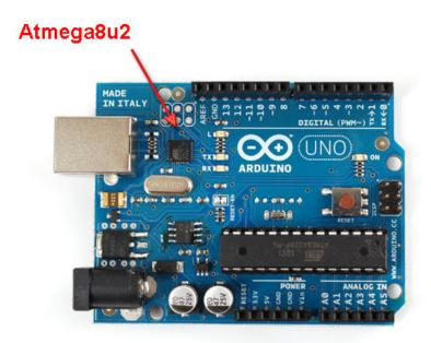
The Uno has changed that by exchanging the FT232RL chip with an atmega8u2 chip. There are a few things that are possible with this new chip but before we discuss that lets make it clear that by default, this chip acts identically to the FTDI chip that it replaces. It's just a USB-serial port!
