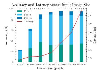
Fig. 5: Accuracy and latency with different input resolutions.
