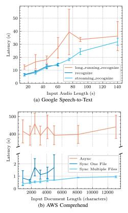
Fig. 3: Latency profiling for three different APIs of Google Speech-to-Text (synchronous, asynchronous, and streaming) and AWS Comprehend (synchronous one file, synchronous multi-file, and asynchronous). Each point in the figure corresponds to the mean and the error bar corresponds to the standard deviation of five experiments. Note that, in (b) the y-axis is broken into two parts with different value ranges.
