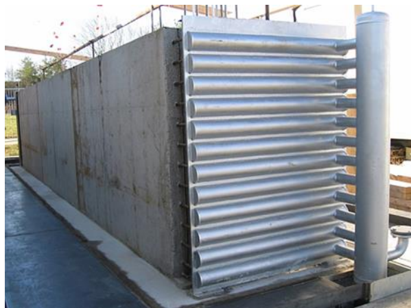
Figure 134: Concrete thermal energy storage. (Reproduced from DLR).
