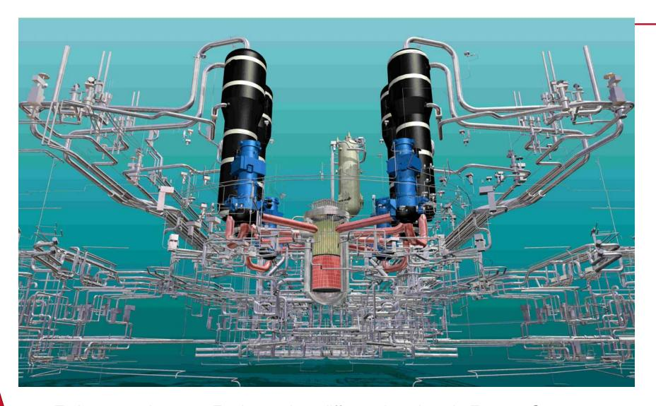
Today more than 200 Engineers in 5 different locations in France, Germany and Finland are designing simultaneously the EPR detailed plant layout in 3D
