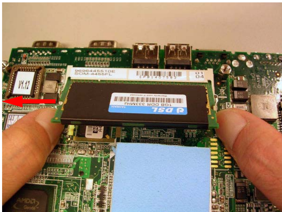
Figure 4.9 Turn over the carrier board and remove the DRAM module
