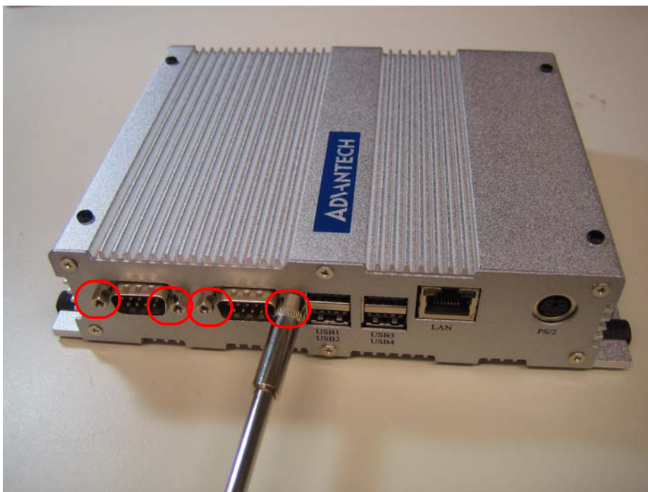
Figure 4.3 Unscrew the 4 Hex-bolt on the front face plate
