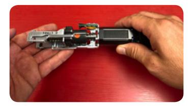
5. Apply Super Lube to top & bottom of post on magnet bracket that will be moving inside of the exit device channel.
