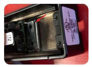
**16.** To find the correct position, pullback on the motor assembly until the it puts a slight tension on the back activating bracket
