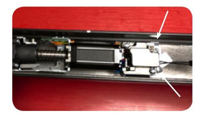
**17.** Tighten both screws while holding motor in correct position.
