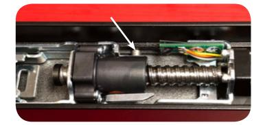
**9.** Now, we're going to hook onto the roll pin on the back activating bracket.
