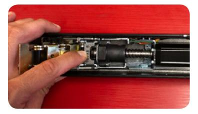
**11.** Next, push down on attaching hooks so they drop down over the roll pin
