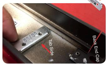
**15.** Drop in both screws into the back of the MM4 bracket but do not tighten yet!
