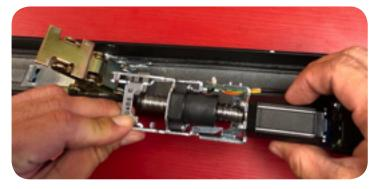
8. Extend Ballscrew all the way until it's touching the built-in stop.
