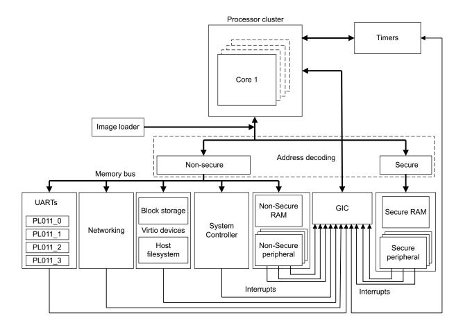
Figure 19-1 Block diagram of ARMv8-A Foundation Platform
