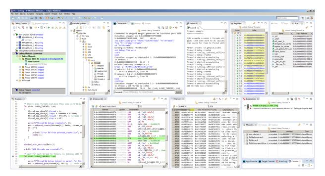
Figure 18-2 Threading call stacks in the DS-5 Debug Control view
