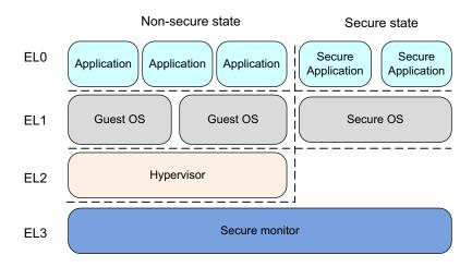
Figure 17-5 Security model when EL3 is using AArch64
