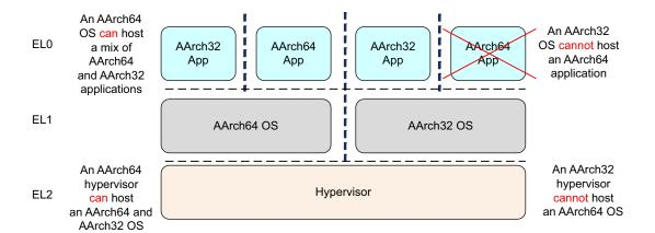
Figure 3-7 Moving between AArch32 and AArch64
