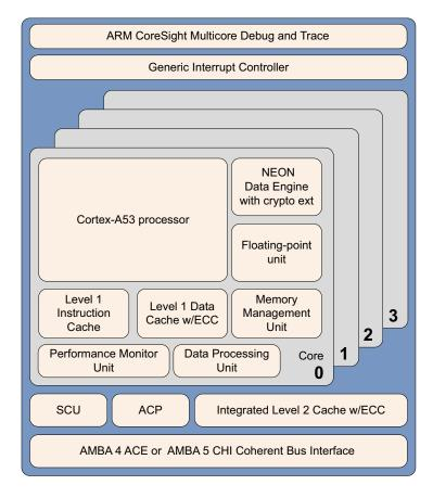
Figure 2-2 Cortex-A53 processor
