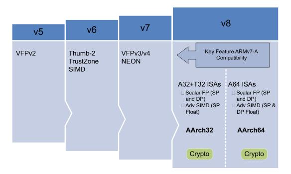
Figure 2-1 Development of the ARMv8 architecture
