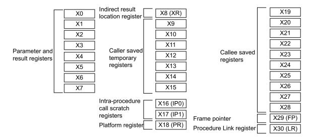
Figure 9-1 General-purpose register use in the ABI
