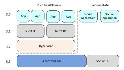
Figure 17-4 Security model when EL3 is using AArch32
