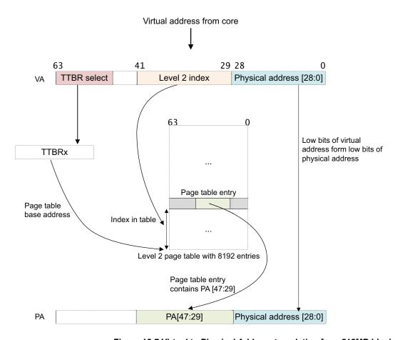
Figure 12-7 Virtual to Physical Address translation for a 512MB block
