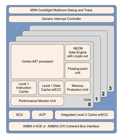
Figure 2-3 Cortex-A57 processor core
