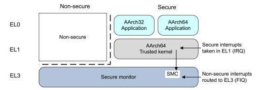
Figure 17-2 Secure interrupts
