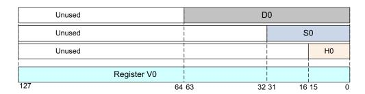
Figure 4-10 Arrangement of floating-point values
