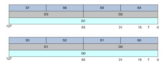
Figure 4-13 Arrangement of ARMv7 SIMD registers
