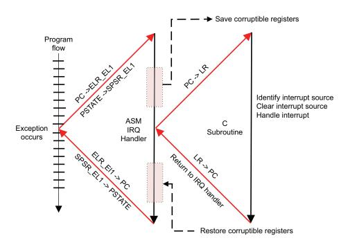
Figure 10-6 Interrupt handler in C code
