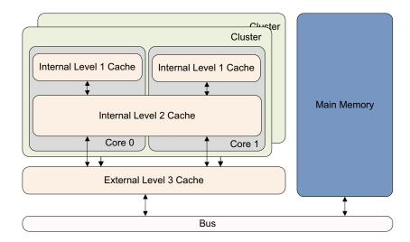
Figure 11-1 A basic cache arrangement
