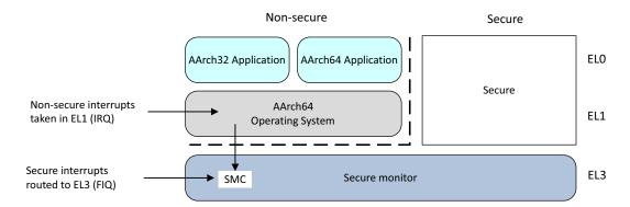
Figure 17-1 Non-secure interrupts
