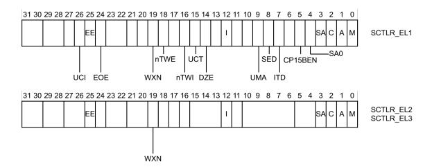
Figure 4-5 SCTLR bit assignments
