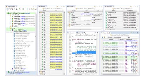
Figure 18-1 Debugging a kernel using DS-5
