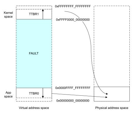
Figure 12-4 Kernel and application memory mapping
