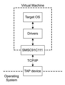
Figure 19-8 Model networking structure block diagram
