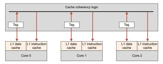
Figure 14-4 Cache coherency logic
