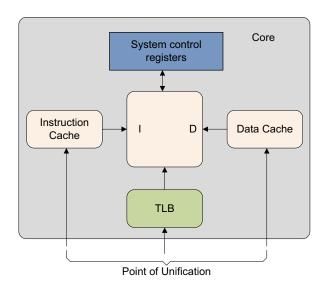
Figure 11-12 Point of Unification
