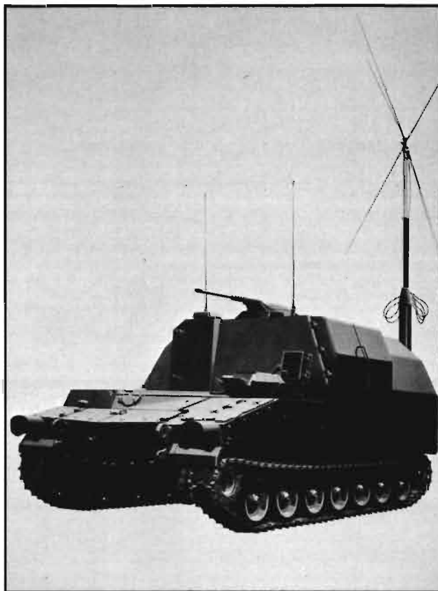
The Command Post Vehicle Test Bed, now under study at Aberdeen Proving Ground, is based on M109-chassis components.
