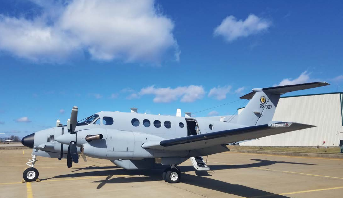
This C-12R Huron is one of the two military variants of the Beechcraft King Air 200 used at the Fixed Wing Army National Guard Aviation Training Site. The C-12R can be modified with EFIS glass cockpit instrumentation for reconnaissance missions.
