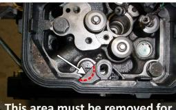
This area must be removed for head stud clearance
