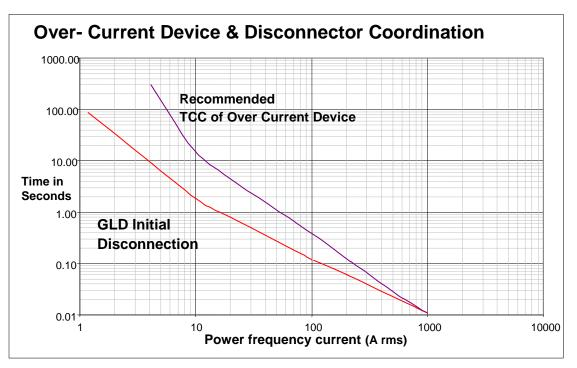
Figure 3 Over-current Device vs. Disconnector Initiation
