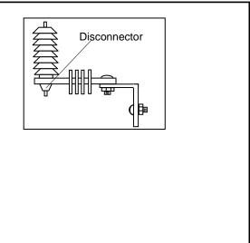
required to operate when an arrester is overloaded and fails.
