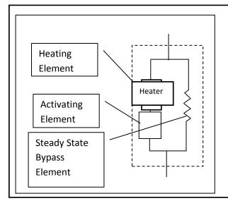
Figure 2 Typical Disconnector schematic
