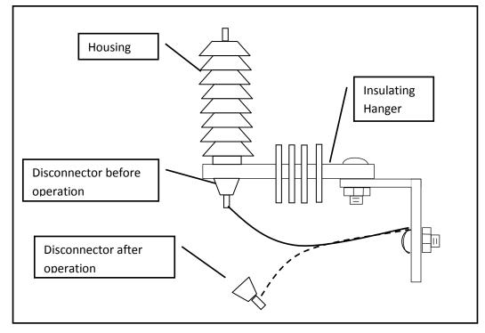
Figure 4 Typical Disconnector Configurations is heated to its activation temperature, it
