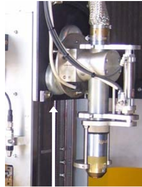
Position of Z Grease nipples under tool head face plate
