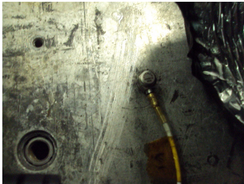
Figure 19: CH 2 Vibration Plate (Z)
