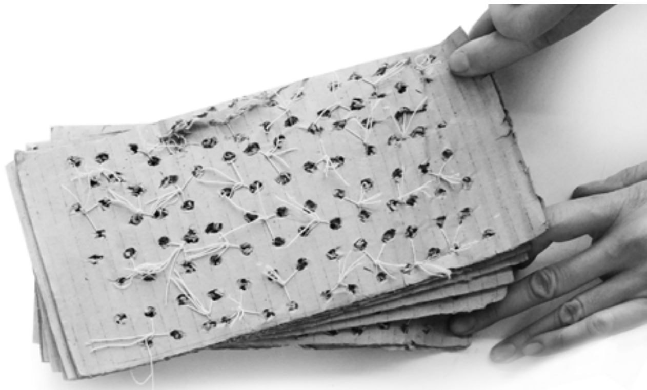
FIGURE 24: Vertical filaments against delamination.
