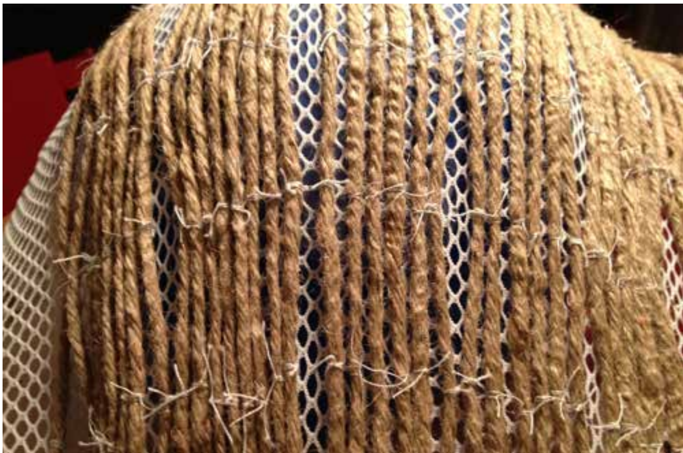
FIGURE 29: Fibres rearrangement after expansion of matrix.. Pores are closed. (Expansion produced by balloon underneath membrane being inflated)
