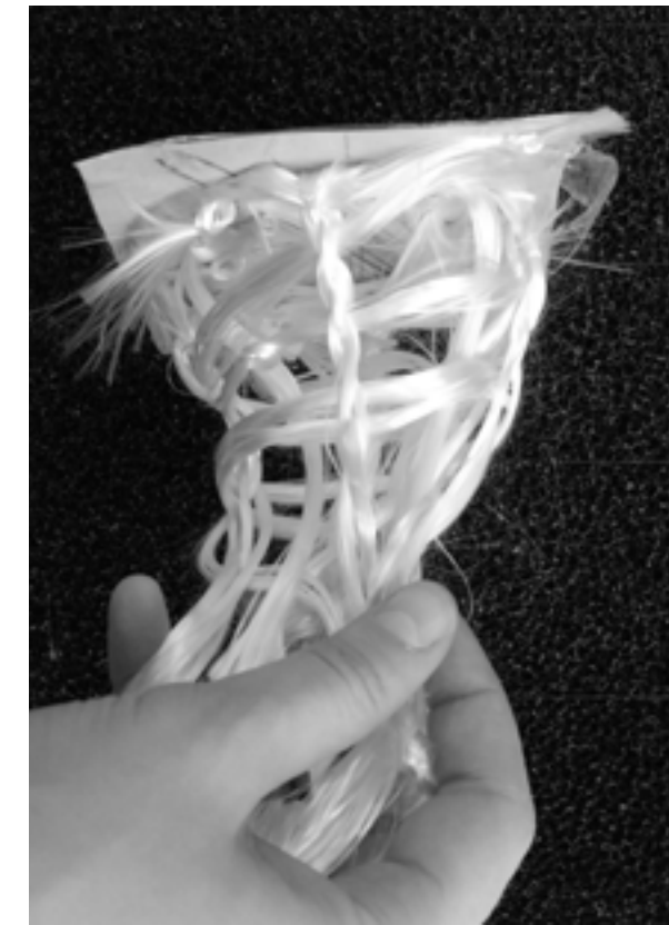
FIGURE 47: Option B. 3D-braiding of pore structures simultaneously with layout of horizontal layers of fibers by Kuka.
