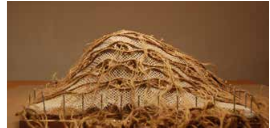
FIGURE 30: Model based on anisotropical stiffness of cuticle. Different layers have been added being treated with different polymers: latex, wood glue, epoxy resin. trying to achieve a multilayered material with different degrees of flexibility. Filaments through the pores are connecting the layers.
