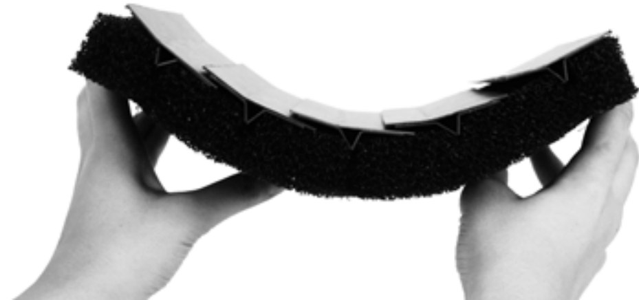
FIGURE 19: Model based on: anisotropic stiffness from inner to outer layers of cuticle.
