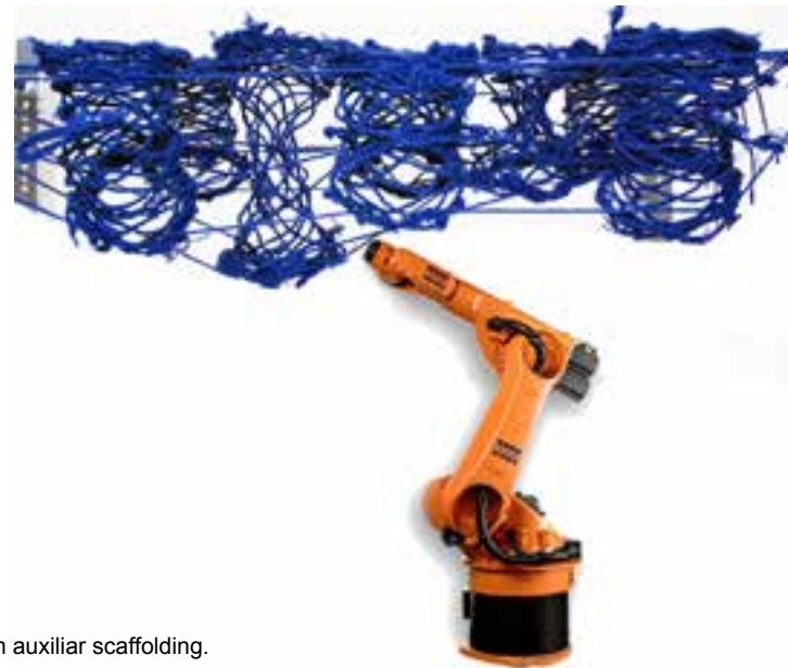
FIGURE 43: Wooden, bamboo or plastic sticks hanging, serving as a guide for the robot.
