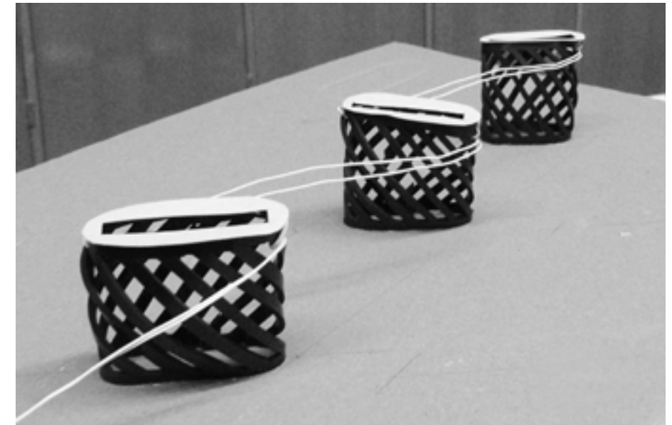
FIGURE 36: Fibers in layers and pore canals direct the way pores close (rotation).
