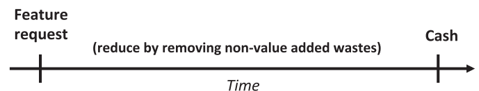
Fig. 1. Lean Thinking aims to reduce the time between order and cash (adapted from Ohno (1988)).
