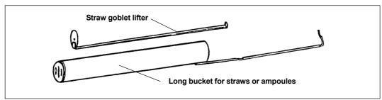
Figure 30. Field bucket and lifter
