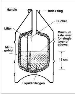
Figure 25. Cross section of a field container
