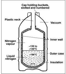
Figure 24. Cross section of a typical semen storage unit.
