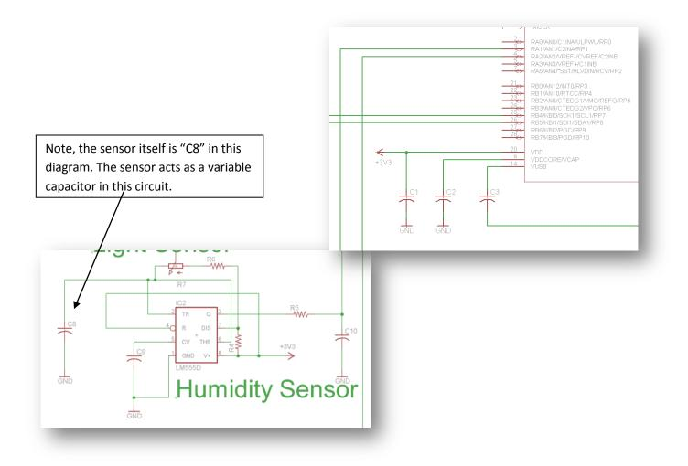
This circuit forces the 555 into an unstable mode of operation. The sensor charges through R6 and R4, then discharges through R6. The microcontroller will read the duty cycle of the output, determined by the capacitance of the humidity sensor (determined by ambient humidity), which will allow us to read the ambient humidity through the microcontroller.
