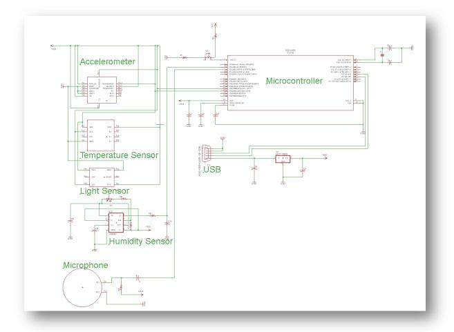
In the schematic above, the accelerometer, temperature sensor, and light sensor are digital devices, whereas the humidity sensor and microphone output analog signals and must be interpreted by the microcontroller.
