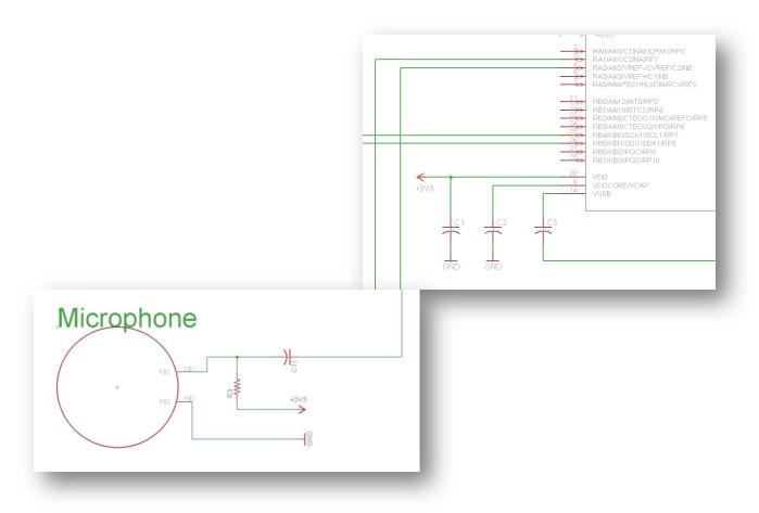
In the following figure, the microphone is acting as a preamp circuit. "C11", above, is a DC blocking capacitor, and the microphone is biased with the power supply. The other port goes to ground:
