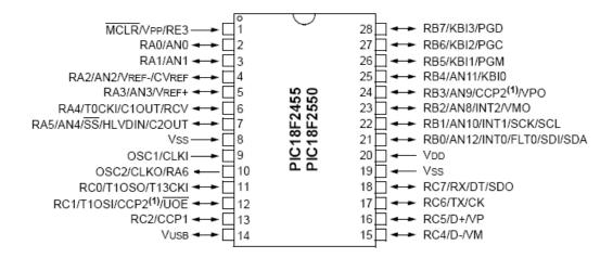
The main reason for this decision was that this device is incorporated with a fully featured Universal Serial Bus (USB) communications module.
