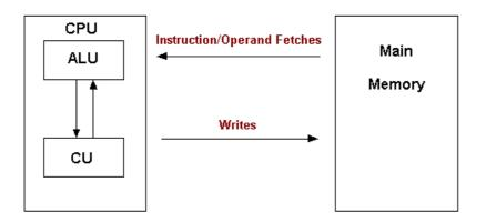
A Von Neumann Machine Schematic
