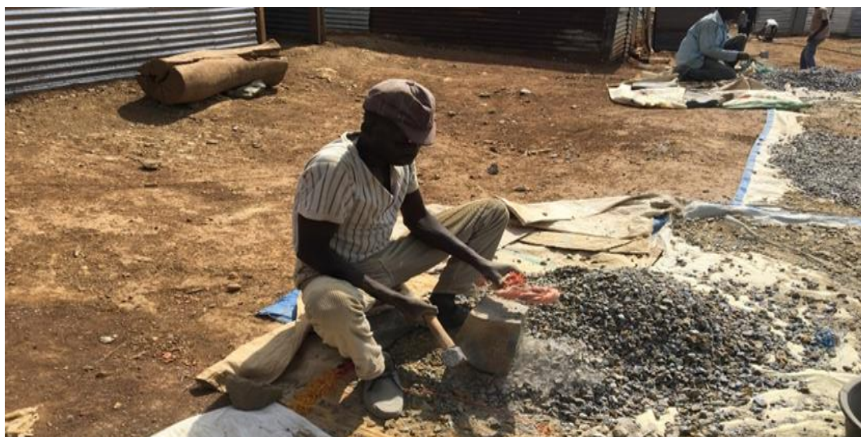
Miner crushing gold rocks by hand stamping at Osiri mine site, Migori.
