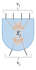
FIG. 1. Schematic of a self-organizing logic gate with internal memory variables,  $\tilde{x}_j$ , that mediate the interaction among the external voltage variables  $v_i$ .
