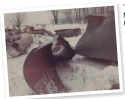
The pipeline operated from November 1, 1968 till December 27, 1968 when there was a blow out in upper Michigan. On January 1, 1969 I was on an airplane to the site to hvdrostatic test the repair. It was -30°F with a 30-mph wind, I was a cold Okie. It blew out 1,200 feet of pipe and it was scrap. Two weeks later it was repaired and during pack it
