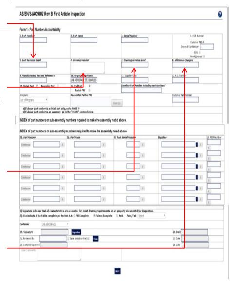
Box 9: Manufacturing Process Reference: The work order number (release/work order number or router number) shall be entered here. See slide 8 for LMI "Synthetic" Part Numbers.
